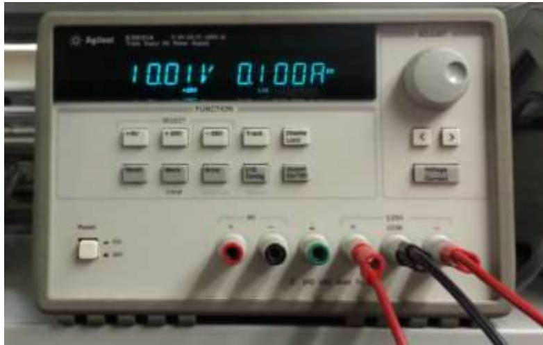
Figure 4 Power Supply. Red cable on the left is +10 V and the red cable on the far right is -10 V. The black cable in between the two red cables is common ground.
